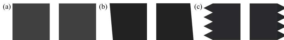
Fig. 7. (a) typical FP cavity with flat surfaces (b) typical FP cavity with tilted surfaces (c) FP cavity with embossed surfaces.
